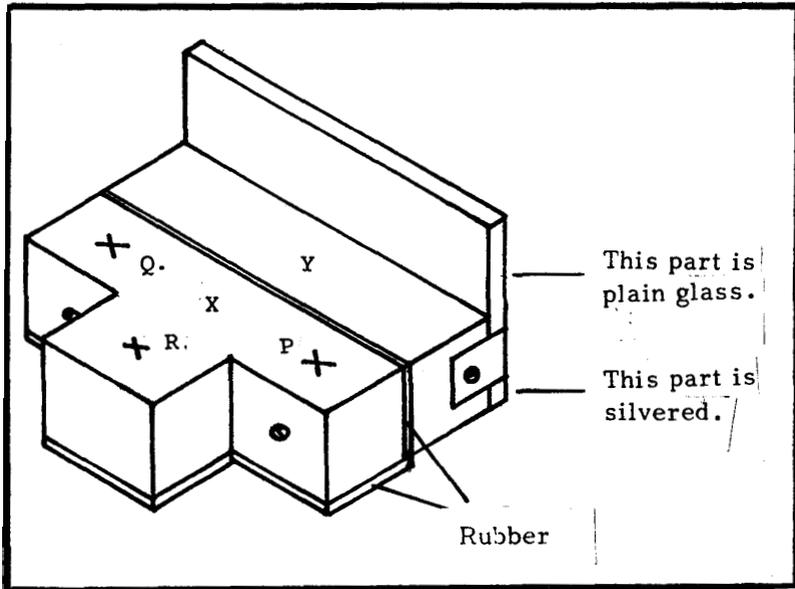
Block "Y" is 2" x  $\frac{1}{2}$ " x  $\frac{1}{2}$ ". The mirror is secured to it with little copper tags as before.
