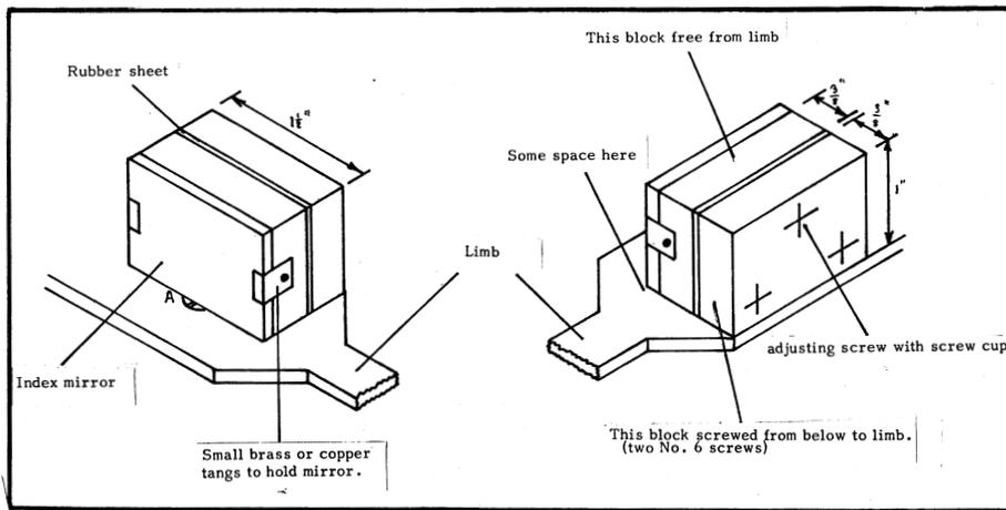
The assembly shown above puts the index mirror parallel to the centre line of the limb which is the simplest position. There are, however, considerable advantages to be got from fitting it at an angle or about  $15^\circ$  to the centre line thus:
